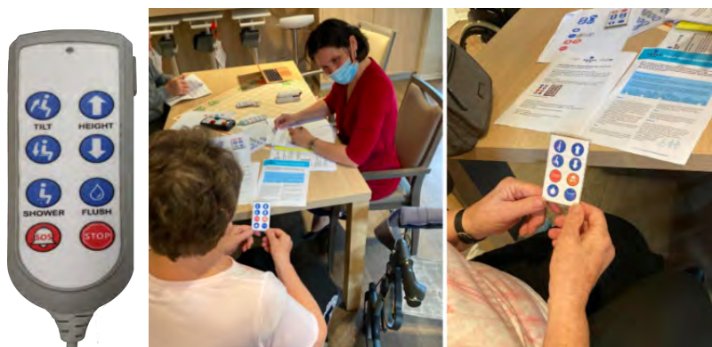
Figure 7. Prototype of the hand control (left) based on findings from co-design activities carried out in 3 European countries (middle and right)
